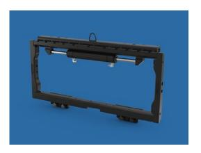
A fork positioner enables the forklift operator to adjust the amount of space between the forks without leaving the seat.
